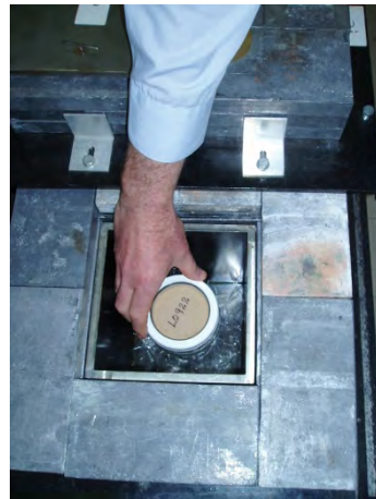
Counting by gamma spectrometry
