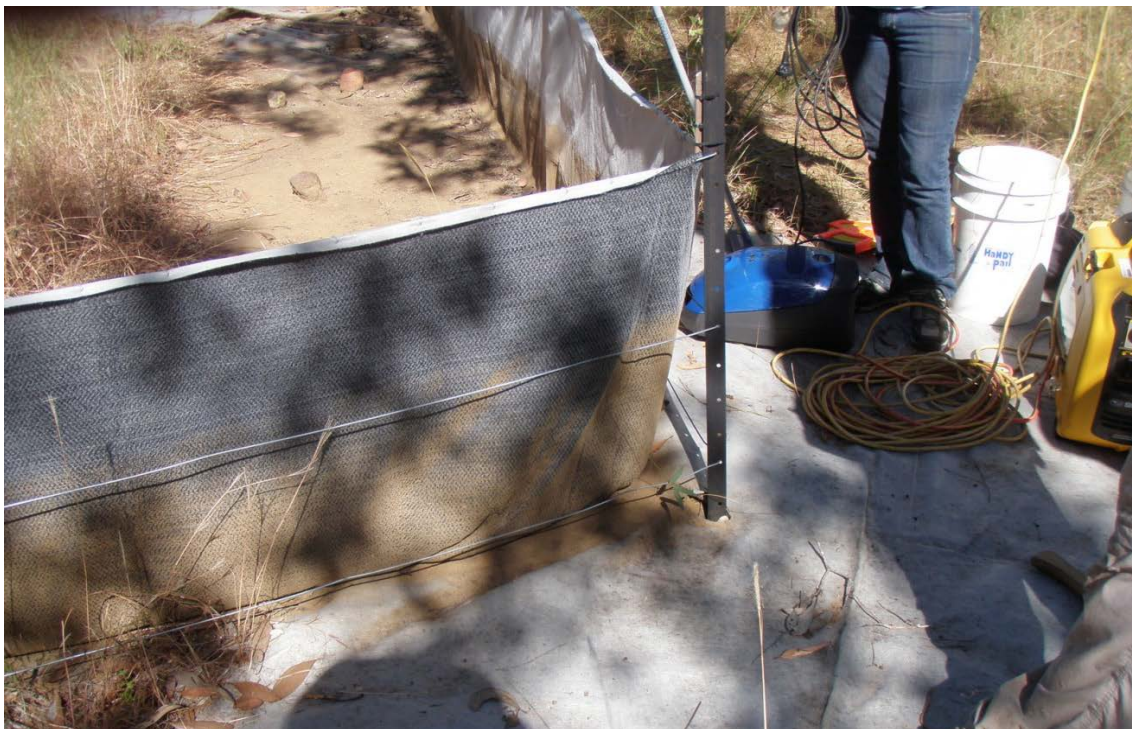
Fine sediment losses through sediment trap geofabric . (Photo: John Spencer)
