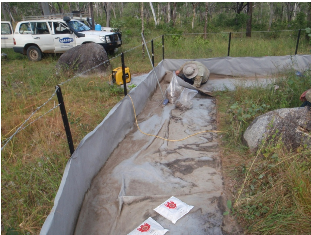
Collecting sediment deposition of 2009–2010 wet season sample from hillslope trap. (Photo: Andrew Brooks)
