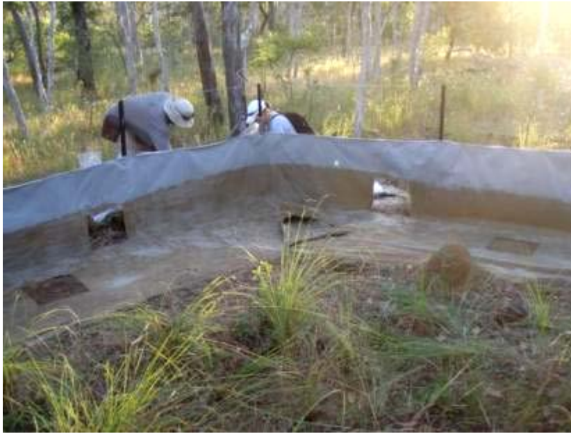
Figure 3 Sediment trap from Normanby sandstone 1, at the completion of the post wet season sediment collection, showing the samples of geofabric taken for analysis of the residual material retained within the geofabric.
