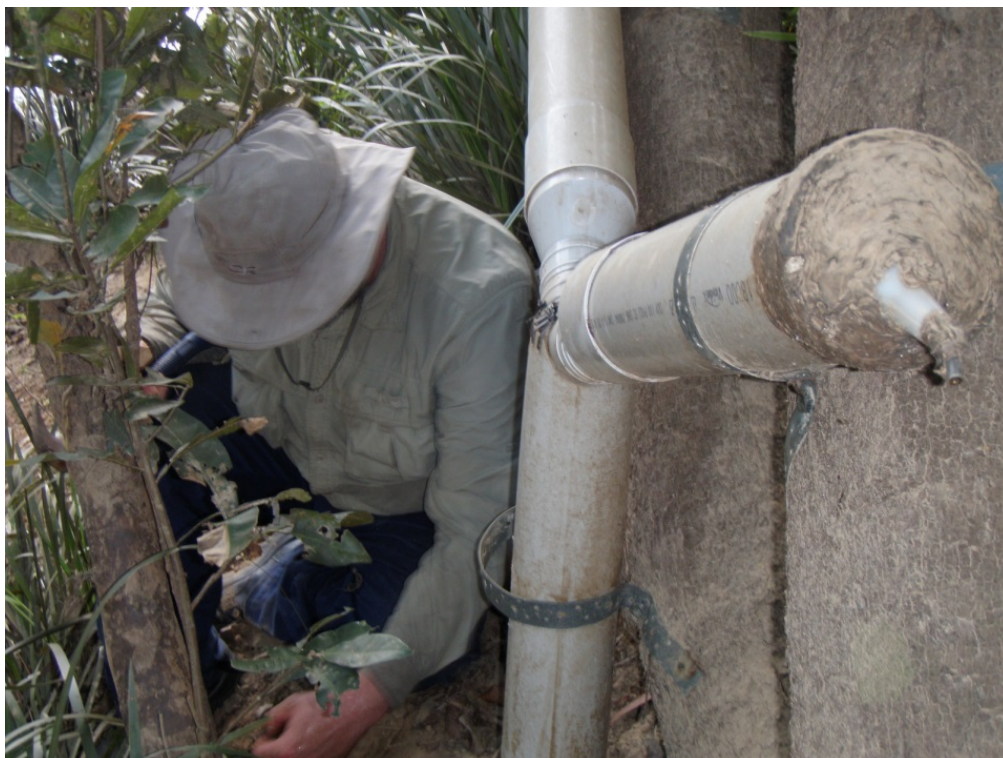
Collecting from Y-integrated experimental sampler at Battle Camp gauge, Normanby River in May, following the 2009–2010 wet season. (Photo: Anne Bourgeault)
