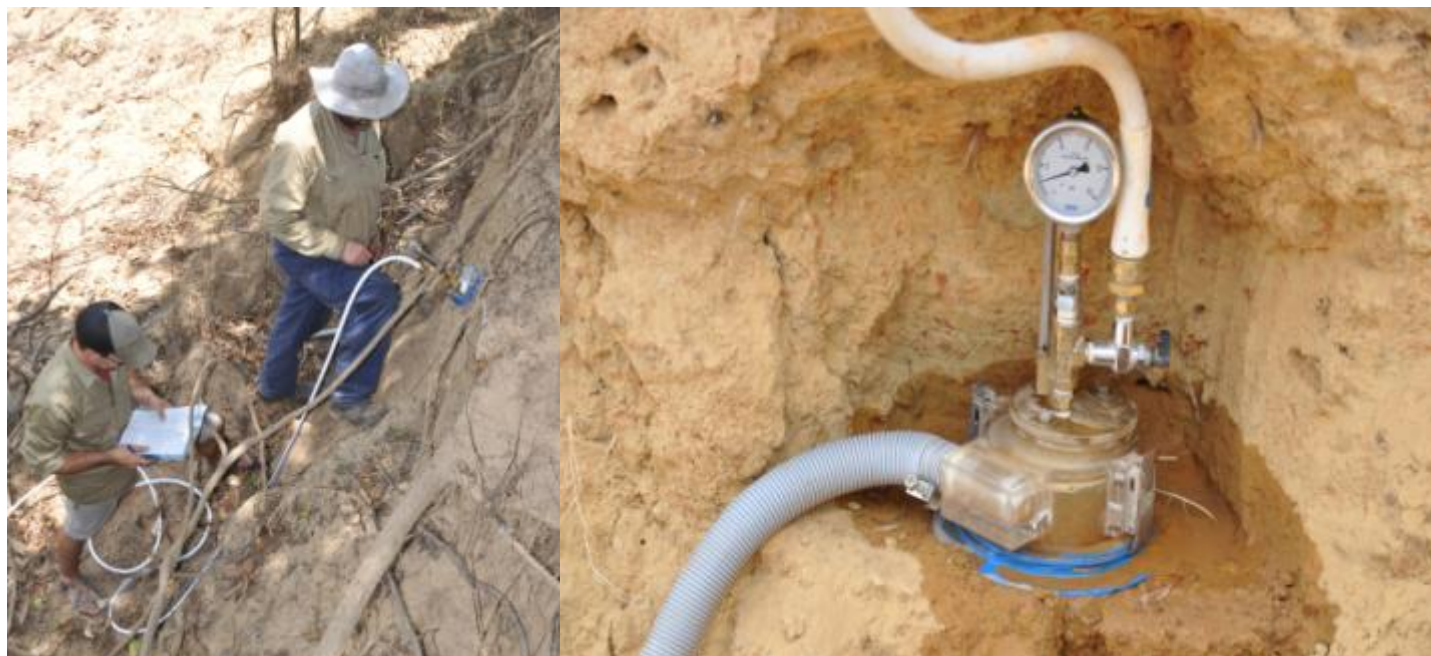
Figure 7 - Conducting jet tests at Normanby 1 and Crocodile Creek
