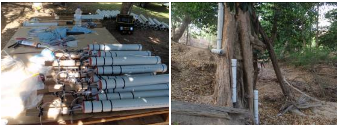
Figure 2 – Left: Rising stage sampler production line – September 2009. Right: Rising Stage Sampler array in the West Normanby River. These samplers collect a suspended sediment sample during the first inundation incident for a given stage. Subsequent inundation episodes are not collected and should not affect the existing sample. A pressure transducer stage recorder at the site allowed the identification of the precise point in the hydrograph that the sample was collected, which was correlated to nearby gauge discharge data.
